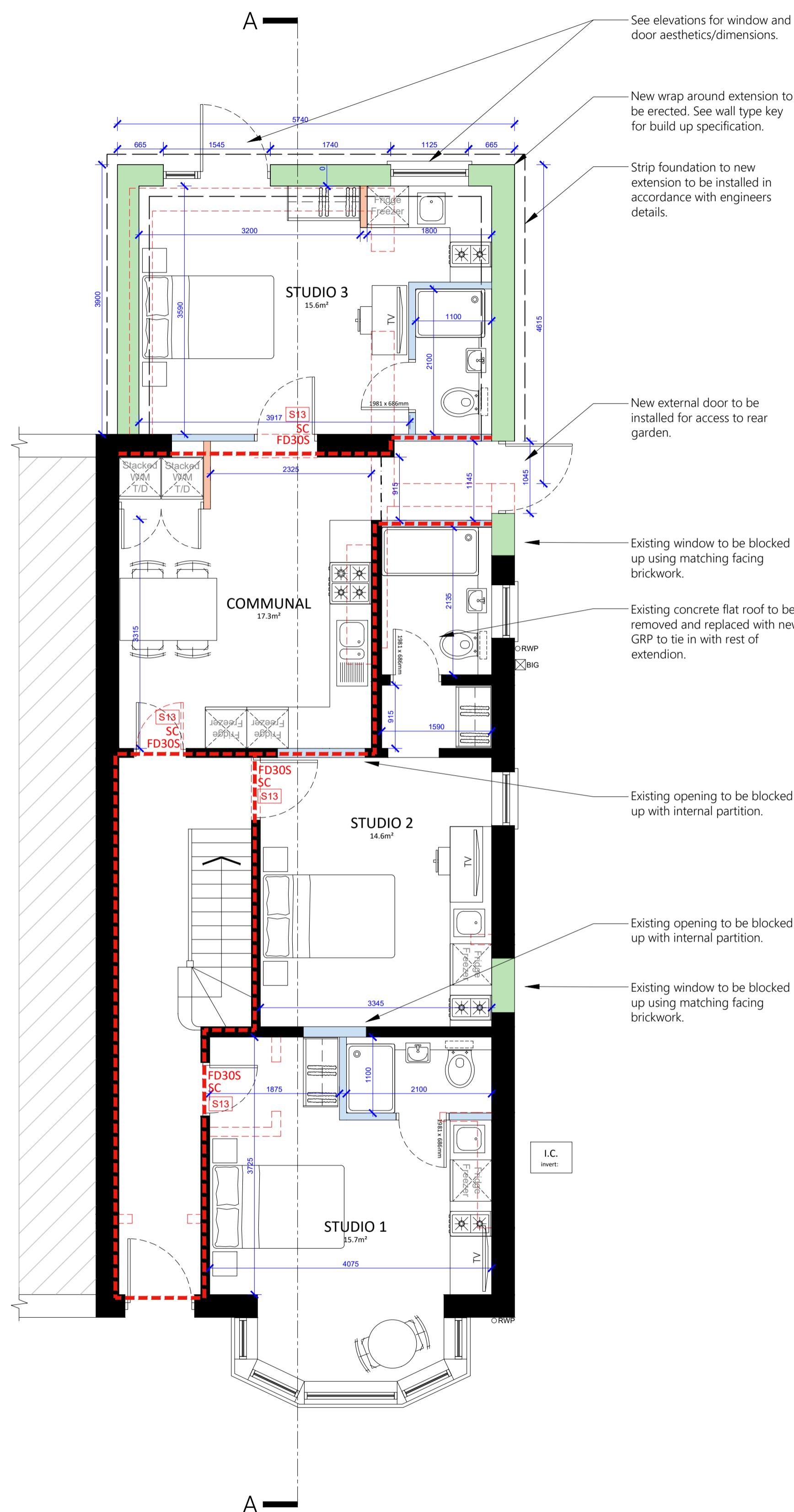
Ground Floor Plan Scale 1:50
